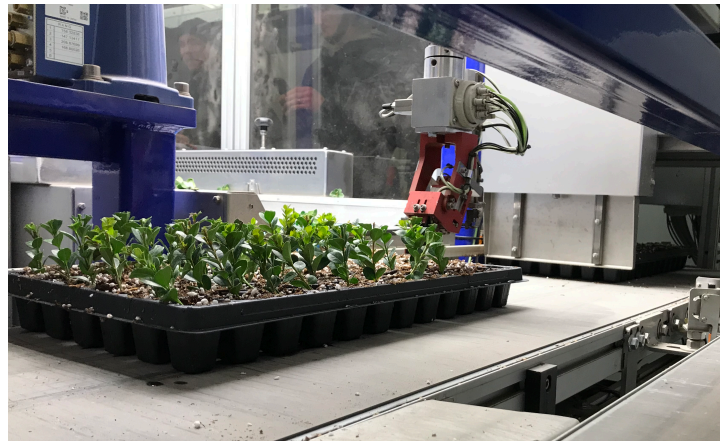
Figure 1. Robotic vegetative cutting machine used to stick vegetative cuttings.
