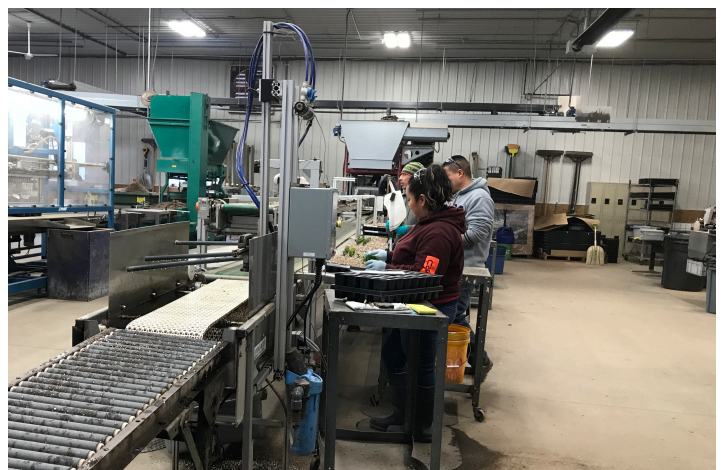
Figure 3. Employees sticking cuttings using the progressive sticking technique.
