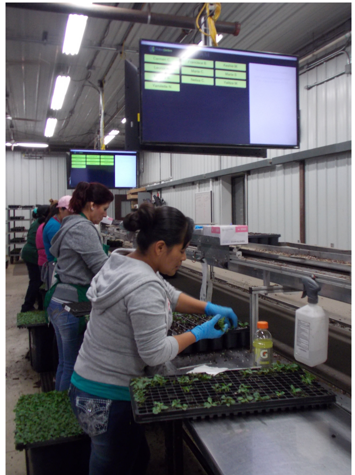
Figure 5. TV monitors above employees sticking vegetative cuttings provide instant feedback to individual employees about their performance.
