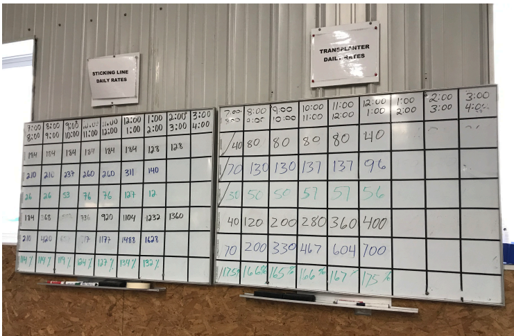
Figure 4. These white boards quickly show employees the hourly sticking rates of the team with respect to their goals.
